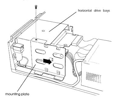
2. Turn the hard disk drive so the components face up and the connectors face left. Then place the mounting plate on the hard disk drive and align the four holes in the plate with the four holes in the drive, as shown below.
